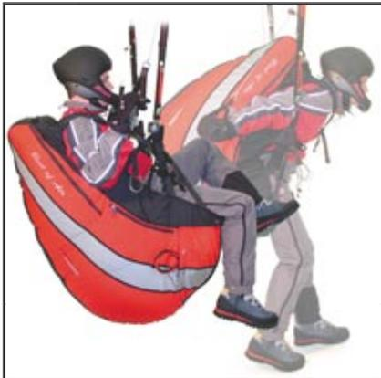
🇬🇧 Especially easy transition to the seated position after launch merely by weight shift due to the special SIL-harness geometry.
